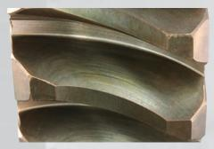
Following severe worm gear testing, RC Series protected gear teeth against wear and corrosion for long life.
